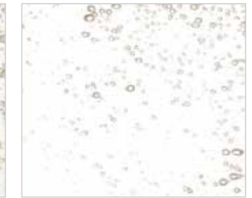
polyalphaolefin (PAO) air release: 12 seconds
