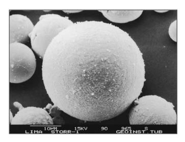
Many particles have a cavity on the one side because of the sudden shrinkage of the metal. If tool steel is used these microscopic balls are often hollow and have sharp edges that can injure the human skin.
