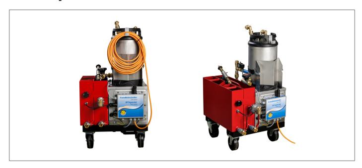
This oil separator is made of stainless steel and sheet steel. The 15 liter tank for separated oil can be removed without tools. The fluid surface is drawn off by suction using a skimmer.
